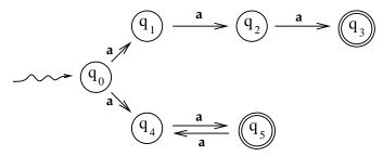
We now apply the algorithm to convert an NFA into an equivalent DFA. Each state of the DFA is a subset of the set of states of M. Since M has 6 states, there are  $2^6 = 64$  such subsets altogether. Fortunately, most of those states are useless, and thus we don't need to include them in our figure. The only ones we show are  $\{q_0\}, \{q_1, q_4\}, \{q_2, q_5\}, \{q_3, q_4\}, \{q_5\}, \{q_4\}$ . In the figure, we abbreviate these names as 0, 14, 25, 34, 5, and 4.
