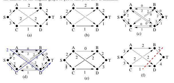
Figure (c) shows the residual graph. (d) shows an augmenting flow of 2, and (e) shows the combined flow, which is 5. (f) shows a mincut of 5, proving that our flow of 5 is maximal.
