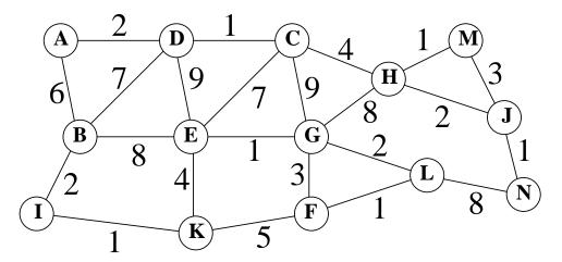
We process the edges in increasing order of weight, using the given tie-breaker. The order of edges is DC, GE, KI, LF, MH, NJ, DA, IB, JH, LG, GF, MJ, HC, KE, KF, BA, ...
