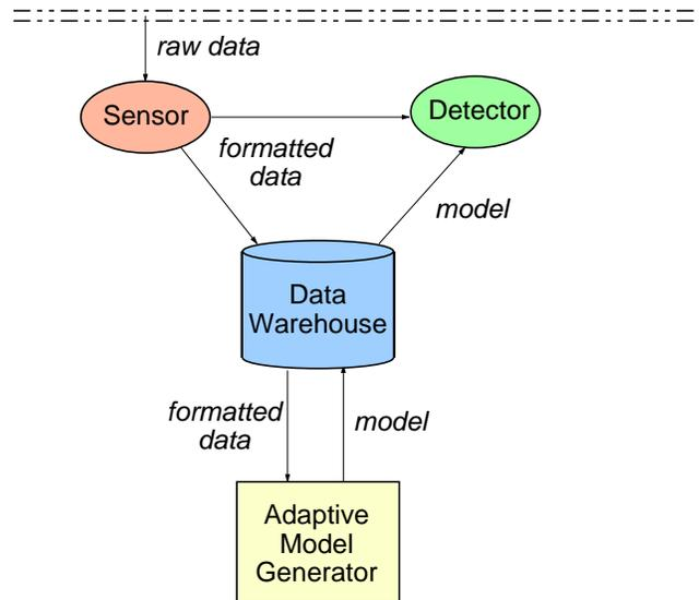
**Figure 2. The Architecture of Data Mining-based IDS**
