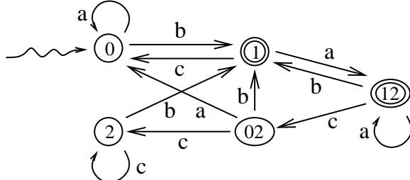
The DFA  $M'$  equivalent to  $M$ . To avoid clutter, the dead state of  $M'$  is not shown. By comparing pairs, it is quickly apparent that no two of its five live states are equivalent.
